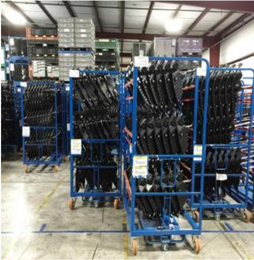
*Stanley Electric racks for the OEM headlight assembly are wheeled into the manufacturing line creating greater efficiency.*
